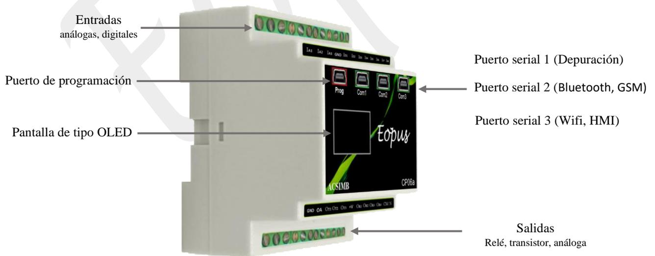
*Figura.1 Estructura PLC CP06a*
